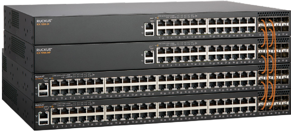
Figure 1: Up to 12 Ruckus ICX 7250 Switches can be stacked together using up to four full-duplex SFP+ h10 Gbps ports for a fully redundant backplane with 480 Gbps of aggregated stacking bandwidth.
